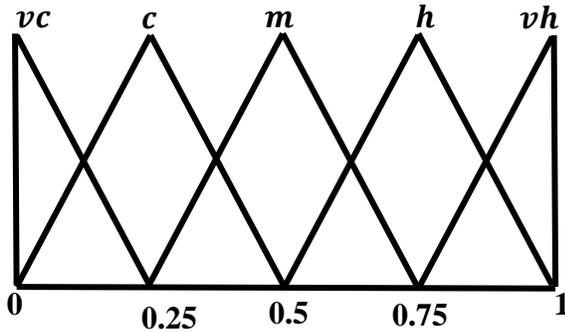
**Figure 3: Triangular membership function representation of 'temperature'**
