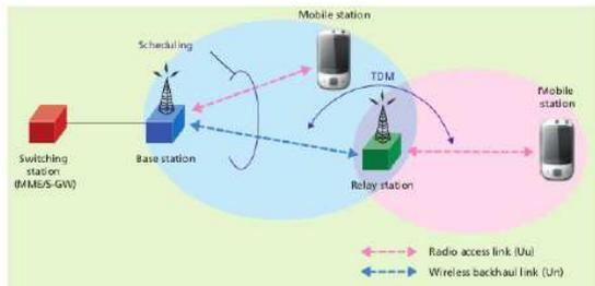
**Figure 1: LTE Relay Network Architecture**
