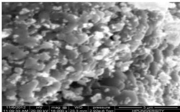
Figure 5 SEM of CuO Nanoparticles
