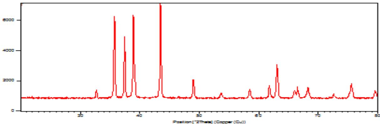
Figure 1 XRD OF CuO nanoparticles at  $600^\circ\text{C}$ (4HRS)
