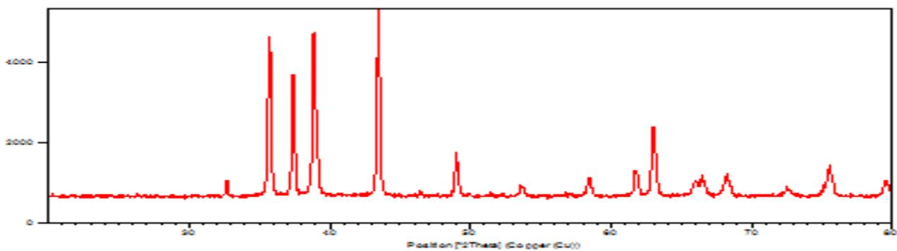
Figure 2 XRD OF CuO nanoparticles at  $600^\circ\text{C}$  (6HRS)
