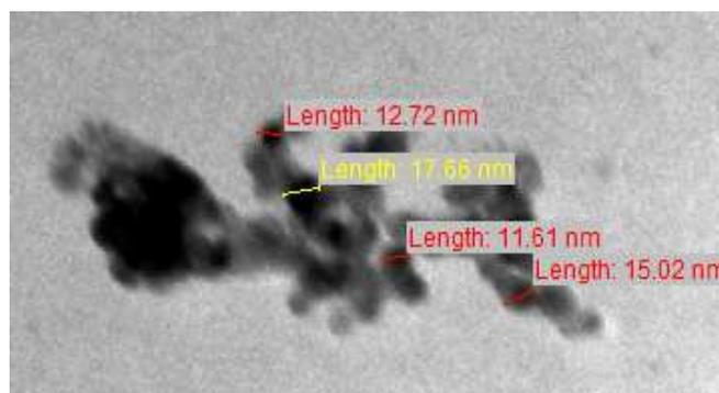
Figure 4 TEM of CuO Nanoparticles
